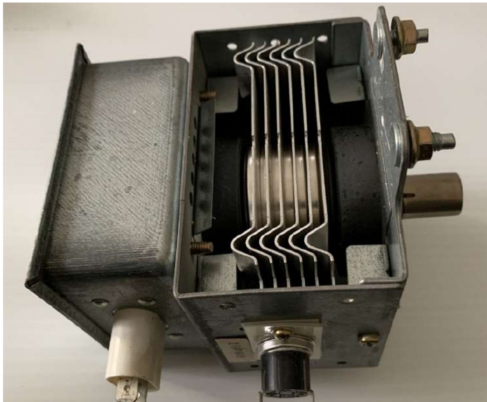
Figure 1. Magnetron used as the microwave electromagnetic-wave source in the laboratory experiment. Original photograph supplied by the researcher.
