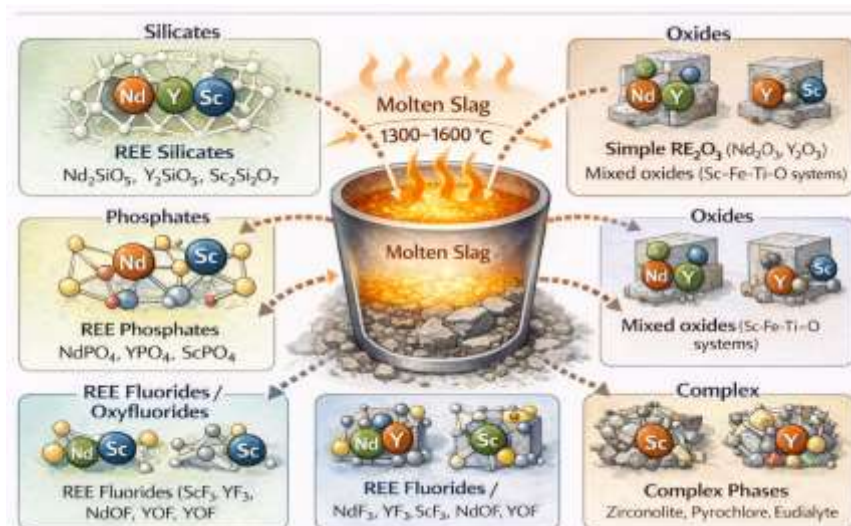
Figure 2. Schematic representation of rare earth element partitioning into silicate, oxide, phosphate, fluoride, and complex phases during high-temperature slag formation (1300–1600 °C). Adapted from Chen et al. (2023) and Gao et al. (2022).
