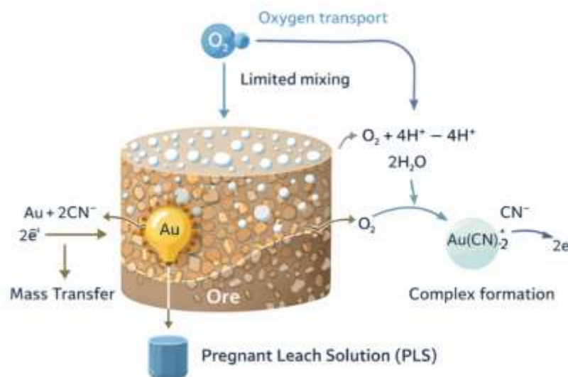
Figure 6. Simplified mechanism of gold dissolution in cyanide solutions, including oxygen reduction and complex formation (adapted from: Manzila et al., 2022; Fedotov et al., 2022).
