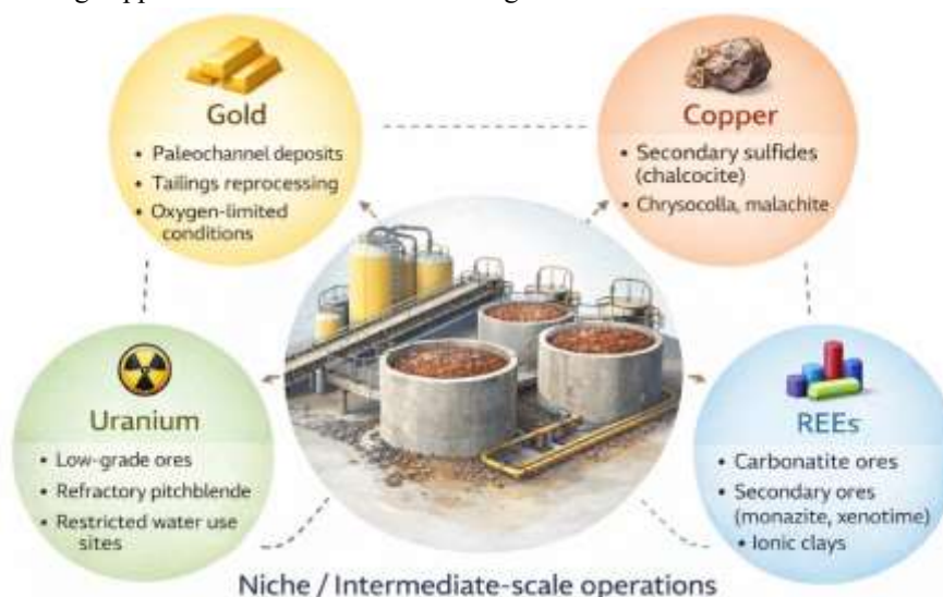
Figure 7. Main industrial applications of vat leaching across commodities, including gold, copper, uranium, and rare earth elements (adapted from Petersen & van Staden, 2025; León et al., 2025).
