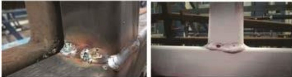
Figure 15: Manufacturing defects that robotized cell intends to prevent using liquid penetrant examination (Castro et al., 2017)
