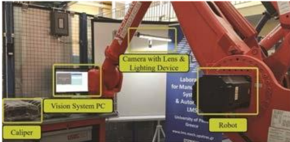
Figure 7. Optical system for quality inspection – experimental setup (Papavasileiou et al. 2021)
