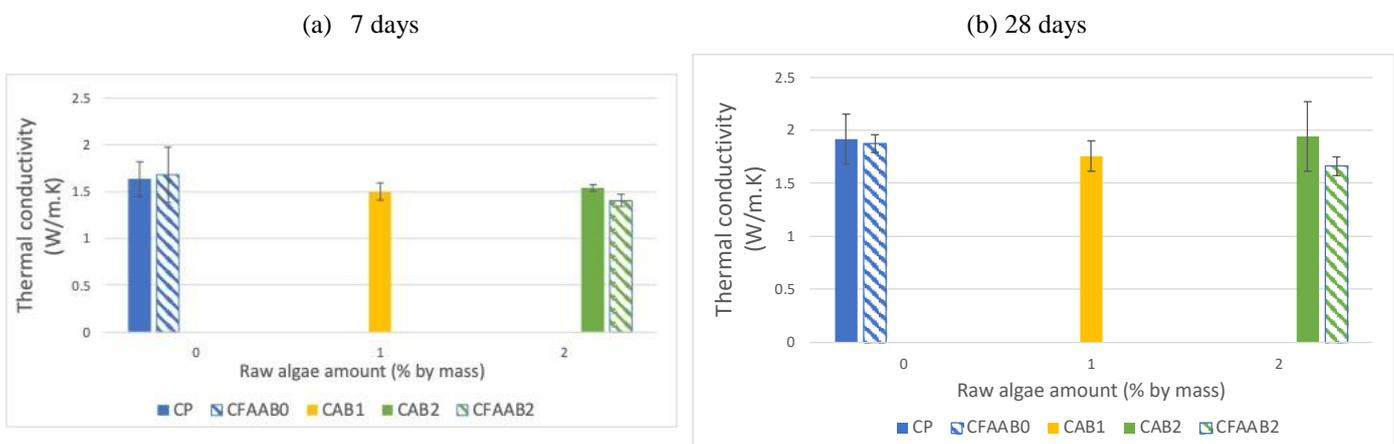
**Figure 7: Evolution of thermal conductivity according to the presence of *Sargassum sp.* as filler and/or reinforcement at 7 days (a) and 28 days (b)**
