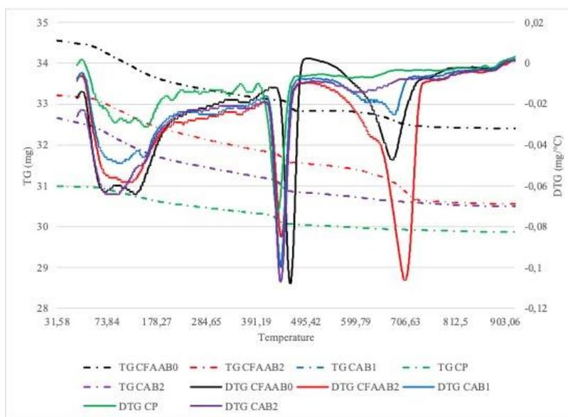
Figure 6: Thermal degradation of cement (CP) and composites
