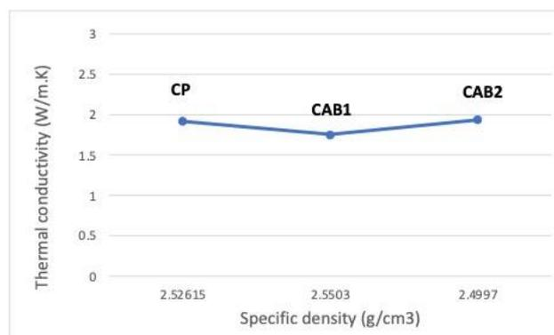
Figure 9: Experimental thermal conductivity according specific density of composites CP, CAB1 and CAB2.
