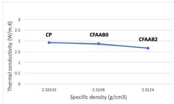
Figure 10: Experimental thermal conductivity according specific density of composites CP, CFAAB0 and CFAAB2.
