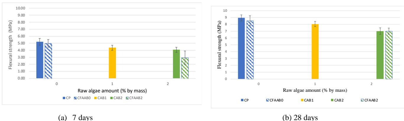
Figure 11: Flexural strength of composites materials at (a) 7 and (b) 28 days
