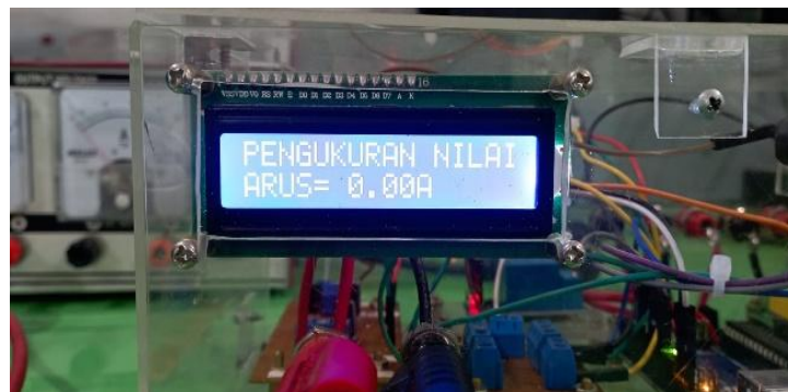
Figure 7. LCD Display When The System Starts The Overcurrent Measurement.
