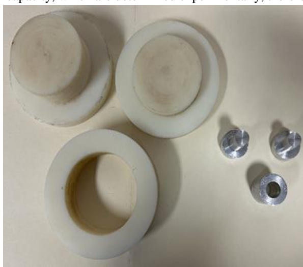
• Figure 3. Models for sargassum tablets to determine thermal conductivity, density, and specific heat
