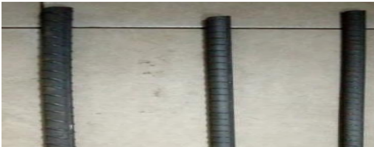
Fig.2. Samples of reinforcement bars of 10, 12 and 16 mm diameter
