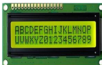
Figure IV. Shape and Pins on a 16x2 LCD [11].
