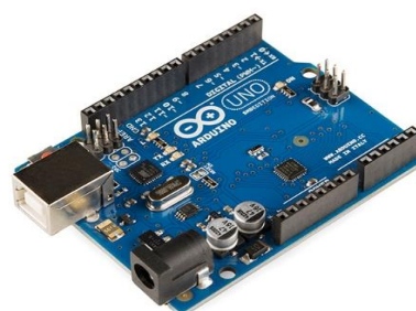
Figure 1. Pins on Arduino Uno [9].
