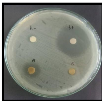
Figure 3: Results of the antibacterial test of silver nanoparticles synthesized using daruju leaf bioreductor
