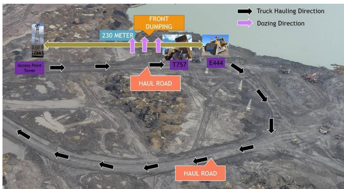
Figure 1. Teleremote dozer trial scheme
