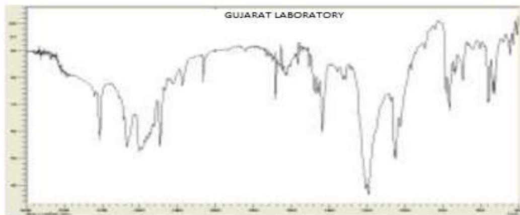
Fig. 2: FTIR spectra of Rasagiline Mesylate and Soluplus
