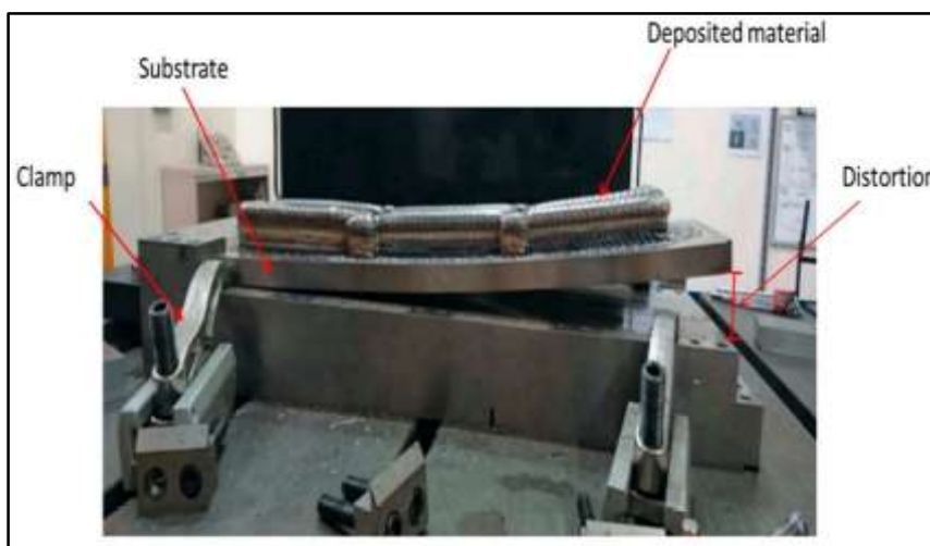
Figure 11. Structural distortion of a WAAM part, as been presented by Xu, F., et al. [17].
