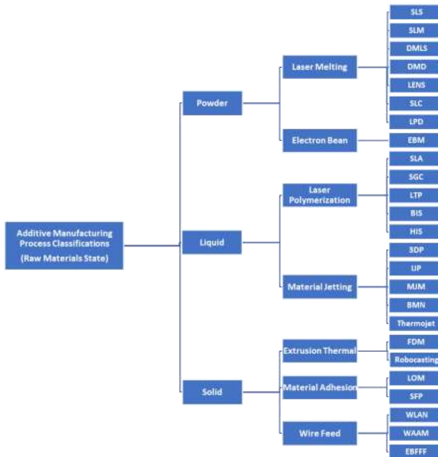
Figure 1. AM process classification depending on the raw material state fed to the system [16].
