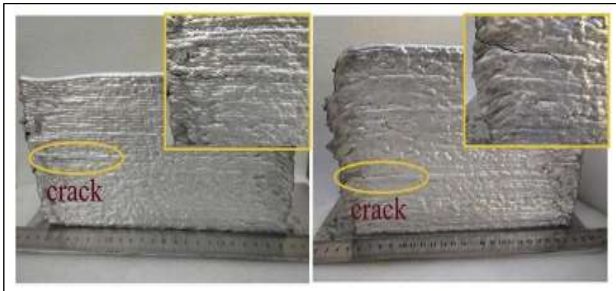
Figure 7. Shows different macrocracks directions on a part of Al 6.6 Zn 2.6 Mg 2.6 Cu alloy produced by WAAM with single-pass multilayers, as presented by Chen, S., et al. [143].
