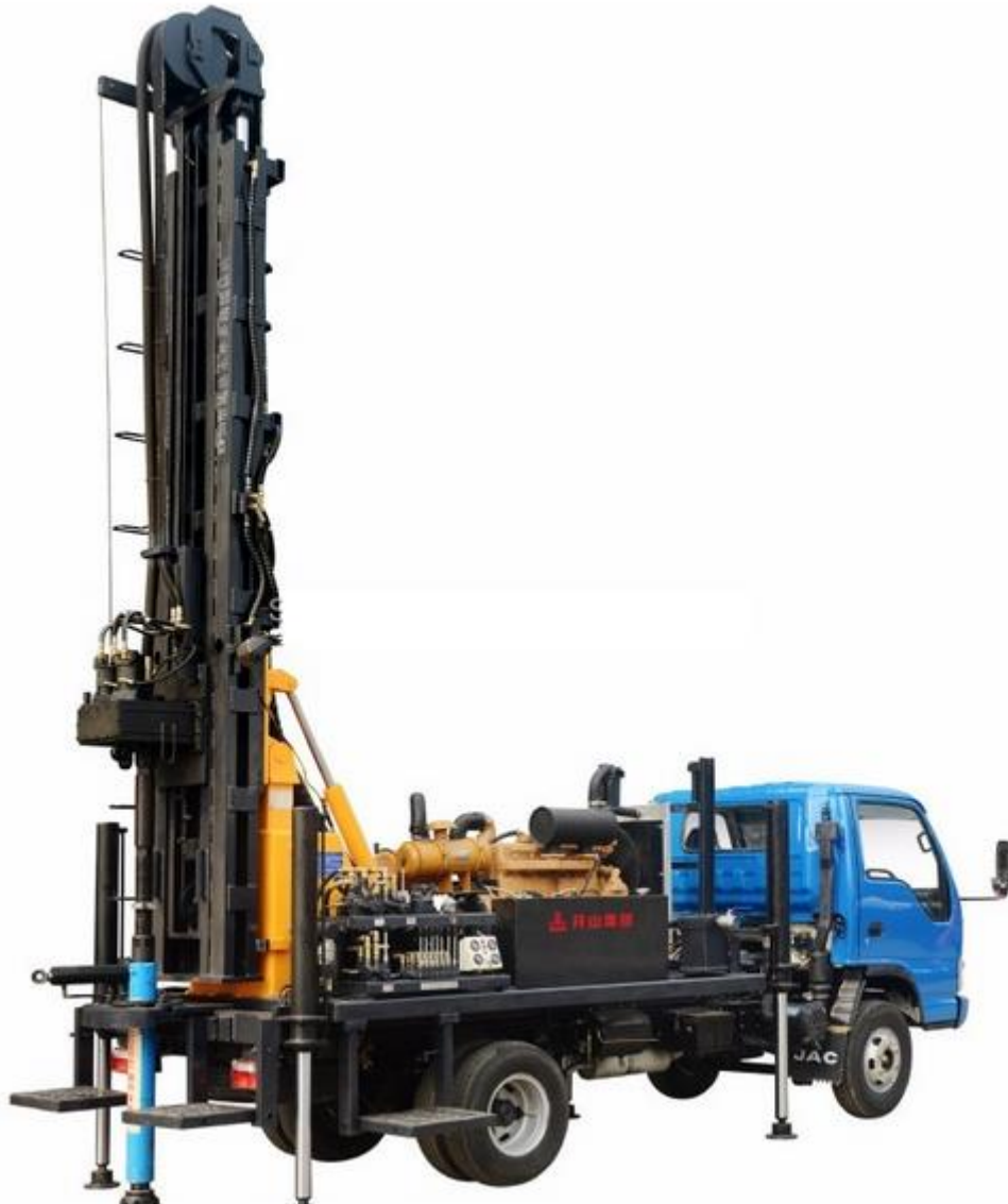
Fig. 5. Rotary Drilling Machine mounted on a Truck
