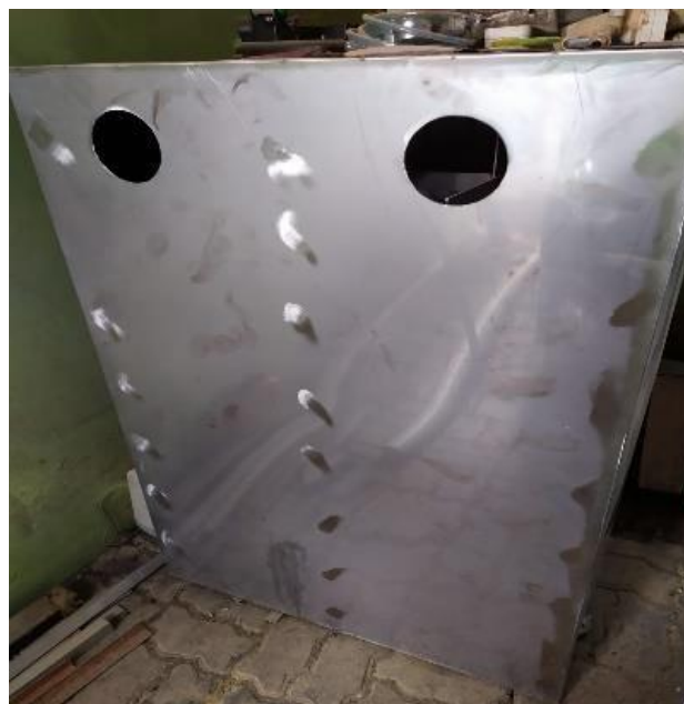
Figure 3. Infiltration well box made of stainless steel
