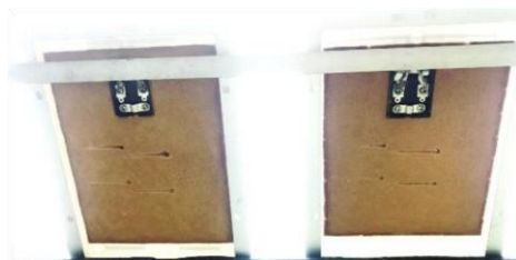
Fig 2. Solar panel after EPCM coating on the back panel at 4 and 7 mm thickness
