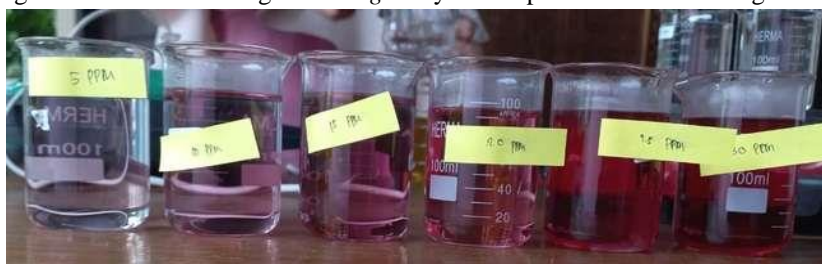
Figure 1. Nanogold synthesis results with concentrations of 5 ppm, 10 ppm, 15 ppm, 20 ppm, 25 ppm, and 30 ppm
