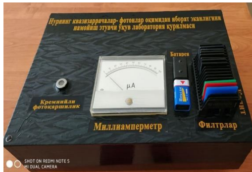
Fig.1. A device for studying the phenomenon of the internal photoelectric effect and its scheme.
