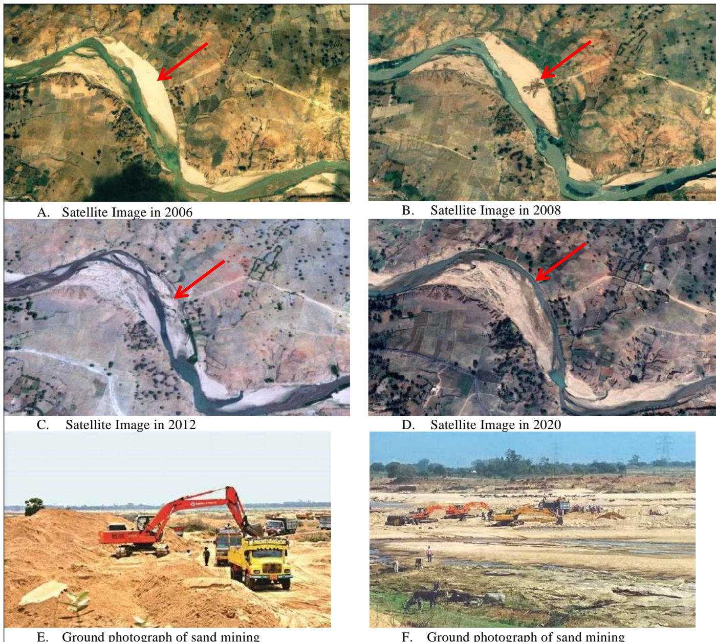
Figure No. 7. Extraction of Sand and has been changed the water flow in river bed.
