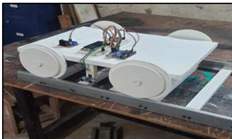
Figure 3: Railway crack detecting system
