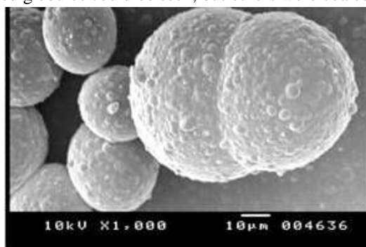
Fig. 3. SEM of Polypyrrole prepared by electrochemical method
